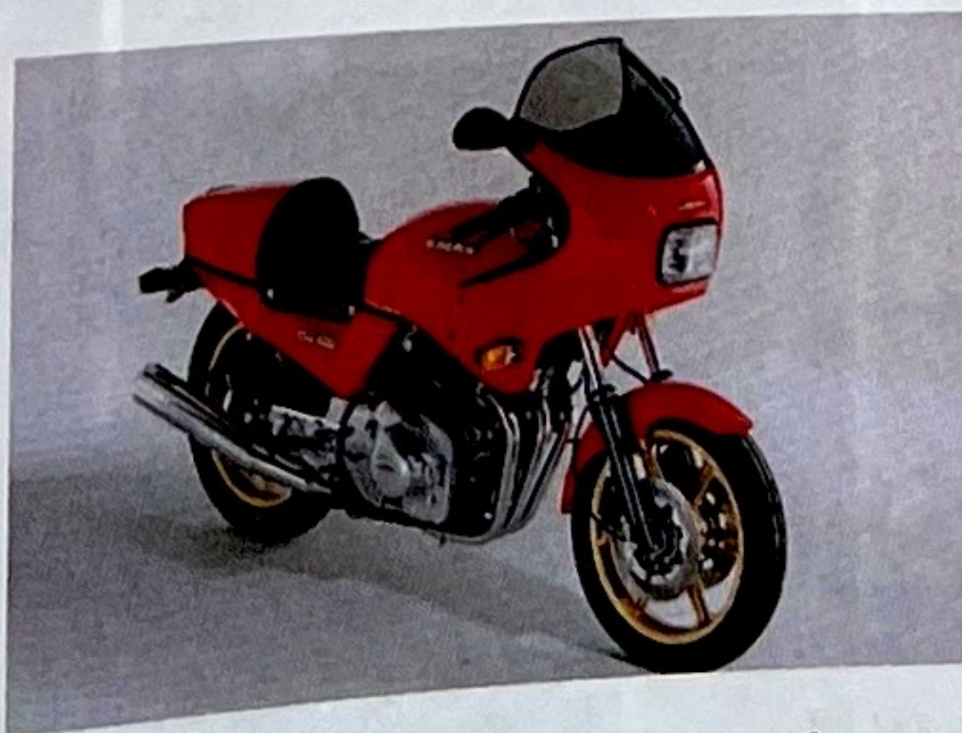
1981 Laverda 1000 RGS – Real Grand Sport. Motorblock in Gummi gelagert, hydraulische Kupplung
